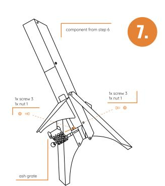
Now insert the grate and secure it with the supplied screws (screw head facing inward, nut facing outward).
