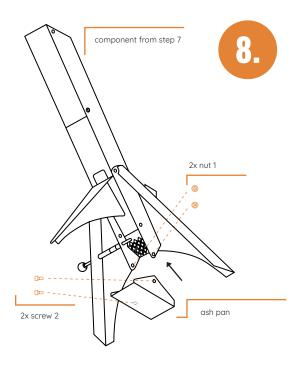
Now attach the ash pan with the lip facing forward (screw head facing outward, nut facing inward; the screw head will later be used as a hinge).
