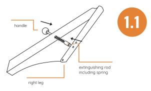
Slide the spring onto the long end of the extinguishing rod and secure it in the base (right leg) using the handle.
