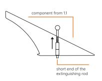
Mount the short end of the extinguishing rod into the base. This is done by compressing the spring.
