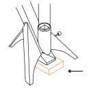
Fix the Pfalzfackel torch with one hand and pull the extinguishing rod evenly and forcefully with the other until all the pellets have fallen out.
