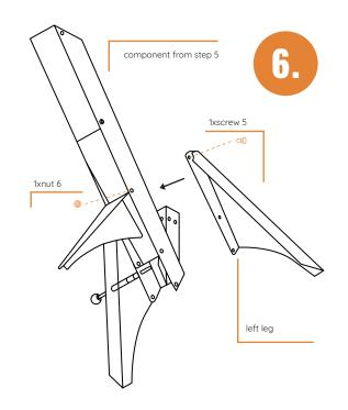
Now attach the left leg (without the preassembled rod) using the top screw (with the screw head facing outward and the nut facing inward).
