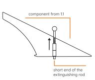
Mount the short end of the extinguishing rod into the base. This is done by compressing the spring.
