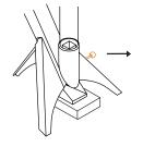
Pull the bowl out from under the Pfalzfackel torch with suitable heat-protective gloves and extinguish the pellets by a stirring motion with a stick or with a little water.
