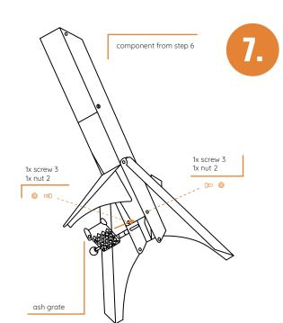
Now insert the grate and secure it with the supplied screws (screw head facing inward, nut facing outward).
