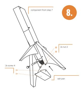
Now attach the ash pan with the lip facing forward (screw head facing outward, nut facing inward; the screw head will later be used as a hinge).
